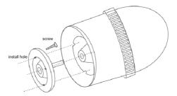
Fix the bottom support to the wall first, then install the unit to support.....
