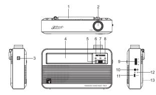
1. Telescopic Antenna 2. Tuning Knob 3. Hand Strap Hole 4. Frequency Indicator 5. Band Selection 6. FM Indicator 7. MW Indicator
